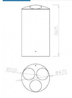
Waste sorting bin made of stainless steel. Matte finish (polished cover). Vandal resistant design. Capacity: 3x50 L. To be placed on the floor. The basket is equipped with three separate containers for segregation in different colors. High quality stainless steel: AISI 304, 1.2 mm. Stickers with inscriptions in Polish language on the cover.
