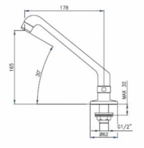
Riser-type washbasin spout with one G1 / 2 connection. The spout&HASH39;s body is made of brass with a layer of chrome. An aerator has been installed at the point of water outflow. The maximum water outflow force may be 21 l/m at a pressure of 3
