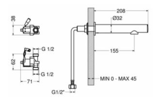
The non-contact 2582 battery is a product that guarantees convenient installation as well as safe and non-contact use. The 2582 battery is a universal product that is suitable for wall mounting - it is worth noting here that it can be attached to a wall such as plasterboard.
