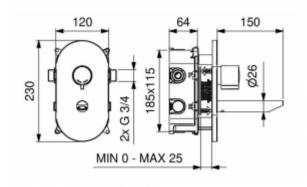
Concealed washbasin tap with built-in mixer. The mixer body is made of corrosion-resistant brass covered with a chrome layer. The 8352 faucet has two G3/4 connections for cold and hot water. A single water outflow, with the standard setting of the faucet, is about 15 seconds ± 3 seconds. The connection pressure can range from 0.5 bar - 6 bar, however, the recommended pressure is 2-4
