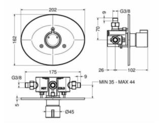
Self-closing flush-mounted mixer with 3/8 &HASH39; connections for cold and hot water, is adapted for wall mounting - shower. The self-closing cartridge is activated by a button built into the central part of the mixer. Temperature adjustment is possible with a lever, the maximum temperature is 38 ° C - setting the min / max temperature in the range of 5-63 ° C is possible only with the use of hydraulic regulation. The whole is made of brass covered with a chrome coating.
