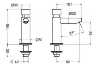
The self-closing basin tap with a moving aerator. The body is made of AISI 316 stainless steel. The tap has one G1 / 2 connection. A single outflow of water takes about 15 seconds (at a water pressure of 3 bar). The amount of water used is 5 l / m. The minimum connection pressure is 1 bar, the maximum is 5 bar. It is worth adding that the recommended connection pressure should be 2-4 bar.
