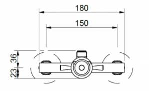
Shower tap with built-in mixer for cold and hot water. The mixer body is made of corrosion-resistant chrome-plated brass. The faucet is equipped with two G3/4 connections for cold and hot water.A single outflow of water lasts 15-25 seconds. Single water flow is 6 l/m, at a connection pressure of 3 bar. The water connection temperature is 5-65°C, while the recommended water connection pressure is 2-4 bar. The 9006MIX/1 tap is available in two options:
