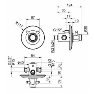
Shower timer with a manual mixer in the form of a rim with protrusions placed around the button, which means that the user has greater control over the temperature of the water supplied even with soapy hands.
