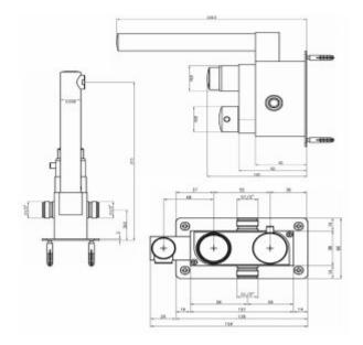
Washbasin timer with thermostatic mixer. Temperature regulation by means of a knob located next to the start button. Possibility of safe water temperature regulation thanks to anti-scalding protection preventing exceeding the permissible temperature of 38 ° C.
