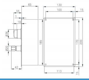
Timed, self-closing mixer used for water supply. The mixer is built into an elegant mounting box, which, apart from the visual value, has a protective nature - AISI 304 stainless steel finish and vandalproof protection. The 9095MIXC mixer is adapted to double 1/2 "connection with the possibility of reduction via a 3/8 &HASH39;half unions. The connection is two-phase, which means that cold and hot water should be connected to the mixer. Moreover, the mixer has a 15-year warranty.
