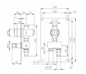
Timed, self-closing mixer used for water supply. The 9095MIXC mixer is adapted to double 1/2 "connection with the possibility of reduction via a 3/8 &HASH39;half unions. The connection is two-phase, which means that cold and hot water should be connected to the mixer.
