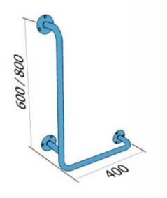
Handrail for the disabled angled right, attached to the wall, 800x400 mm long, made of 25 mm diameter carbon steel tube, powder-coated white. We use this type of handrail in the shower and toilet area. The distance of the handrail from the wall to the center of the tube is 90 mm.
