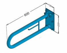
Handrail for disabled people, arched, tilted, a wall with space for toilet paper, 600 mm long, general-purpose, made of 32 mm diameter carbon steel tube, powder-coated, white. We use this type of handrail in the wc area.
