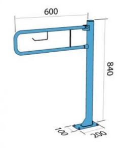
Arched handrail for people with disabilities, floor mounted. With space for paper. 600 mm long, general-purpose, made of 25 mm diameter carbon steel tube, powder-coated in white. We use this type of handrail in the wc area.
