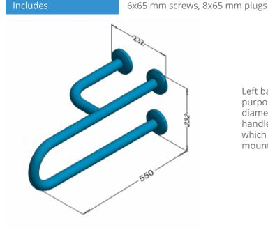
Left basin handrail for disabled people, 550 mm long, generalpurpose, made of polished or matt stainless steel tube, 32 mm diameter. We use this type of handrail in the washbasin. The handles are equipped with masking rosettes with a click system, which allows mounting the masking rosette without the use of mounting glue.
