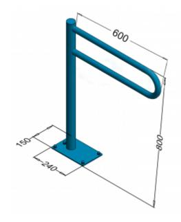
Fixed arched floor railing for disabled people, length 600 mm, general-purpose, made of polished or matt stainless steel tube 32 mm diameter. We use this type of handrail in the washbasin, shower, and toilet area.
