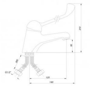
Medical faucet for hot and cold water. Used in outpatient clinics, doctor&HASH39;s offices and hospitals. Thanks to the use of a long lever that facilitates starting and regulating the water temperature, it works great as a surgical bathroom or gastronomy equipment.
