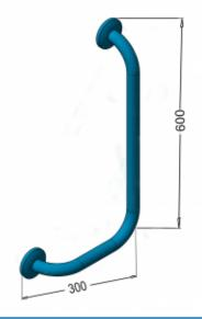
Left angular handrail for disabled people, 300 x 600mm long, generalpurpose, made of polished or matt stainless steel AISI 304 tube, fi 32mm. We use this type of handrail in the washbasin, shower, and toilet area. The handles are equipped with masking rosettes with a click system, which allows mounting the masking rosette without the use of mounting glue. The distance of the handrail from the wall to the center of the tube is 90 mm.
