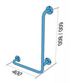
Handrail for the disabled, angled left, attached to the wall, 800x400 mm long, made of 25 mm diameter carbon steel tube, powdercoated white. We use this type of handrail in the shower and toilet area. The distance of the handrail from the wall to the center of the tube is 90 mm.
