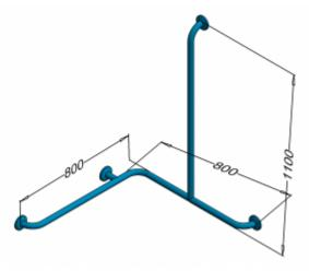
Left angular handrail for disabled people, 800 x 800 x 1100 mm long, general-purpose, made of polished or matt stainless steel tube, fi32mm. We use this type of handrail in the washbasin, shower, and toilet area. The distance of the handrail from the wall to the center of the tube is 90 mm.
