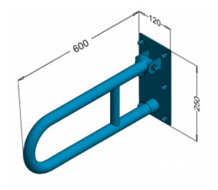
Arch hand-tilt, wall, for disabled people, 600 mm long, generalpurpose, made of polished stainless steel tube or matt 32 mm diameter. We use this type of handrail in the washbasin, shower, and toilet area.
