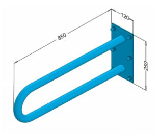
Arch fixed wall for disabled people, length 600 mm. general purpose, made of polished stainless steel tube or matt 32 mm diameter. We use this type of handrail in the washbasin, shower and toilet area.
