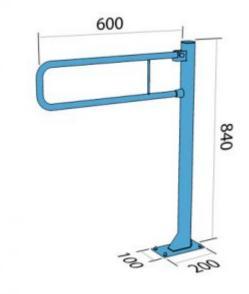
Handrail for disabled people, arched, fixed, floor-mounted, 600 mm long, general-purpose, made of 25 mm diameter carbon steel tube, white. We use this type of handrail in the washbasin, shower, and toilet area.
