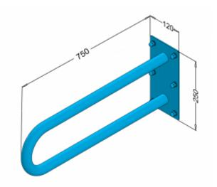
Arch fixed wall for disabled people, length 750 mm. generalpurpose, made of polished or matt stainless steel tube 32 mm diameter. We use this type of handrail in the washbasin, shower, and toilet area.
