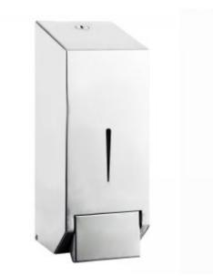
Horizontal liquid soap dispenser in a stainless steel housing. In the middle of the dispenser there is a plastic soap cartridge with a capacity of 1 L, which prevents damage to the container housing - refilling is done by adding soap from the collecting container. Matt surface finish (brushed steel). The infusion is opened by a special key attached to it. It does not require expensive soap refills. On the front of the dispenser is a window to view the amount of soap.
