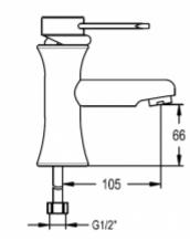
Basin mixer with one G1 / 2 connection for cold or mixed water. The faucet body is made of brass covered with colored epoxy paint. The offered children&HASH39;s battery is equipped with the Eco-Stop system. The mentioned system is a two-stage activation of the water flow. The first activation (tilting the handle to start the battery) stops at a maximum flow of 3 I / m, the second activation (further tilting the handle) increases the maximum water flow to 6 I/m.
