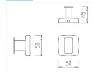
Bathroom hanger. Fastened to the wall with screws. Made of stainless steel. Finish: matte or polished (gloss).
