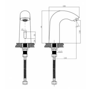
Electronic basin faucet. It can be connected to hot, cold or mixed water. High-quality materials used for the production of time batteries ensure its long-term, trouble-free operation, and also make it extremely vandal-proof. Designed for public utility rooms.
