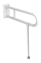
Handrail for disabled people, arched, tilting, wall-mounted, length 800 mm, general-purpose, made of 32 mm diameter carbon steel tube, white powder coated. We use this type of handrail in the washbasin, shower, and toilet area.
